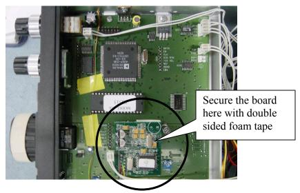
It is convenient to run the wires to the other side of the board through the gap between the panel and the board:
