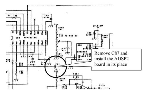
Connect the signal path as shown in the diagram. Your installation should look like this:
