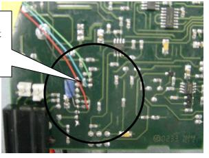
12 VDC can be taken from any point where it is convenient and the ground can be connected to any convenient point that is connected to the chassis ground. Connect the 12 VDC and GND wires from the ADSP<sup>2</sup> board and connect them to the Argonaut's power supply. A convenient location is shown on the schematic below.
